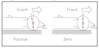
NB: red steering axis, the black vertical to the ground through the point grounding of tyre.
